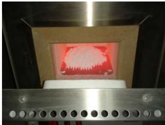
Gambar 1. Proses kalsinasi kalsit Puger
