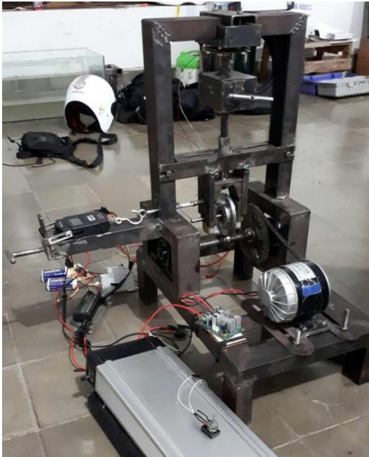
Gambar 2. Alat Uji Rolling Resistance Bearing
