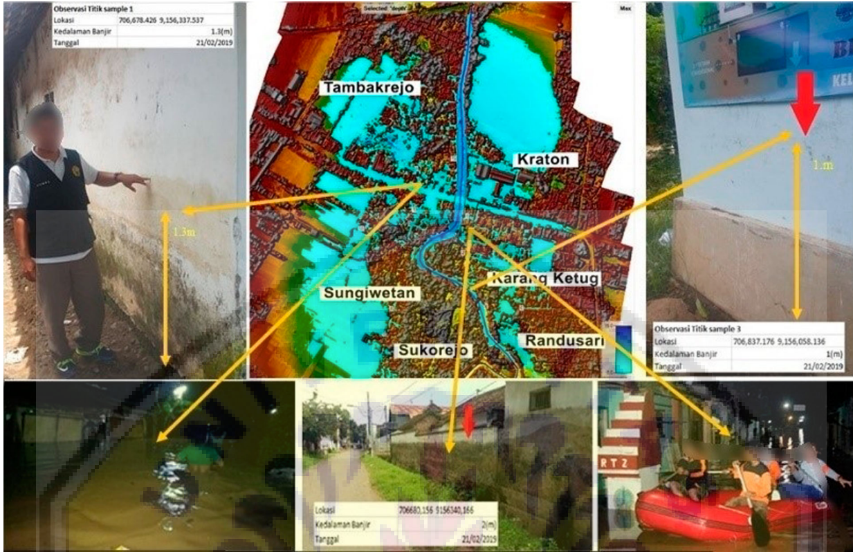
Figure 6. Calibration of Flood Inundation Depth.
