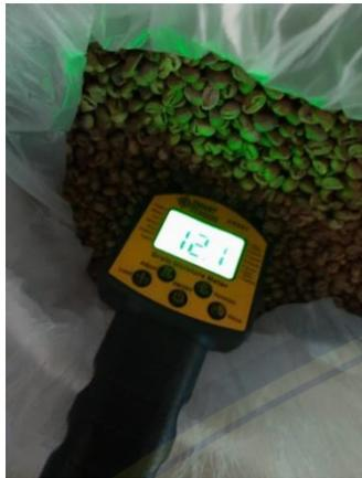
Gambar 1. Pengukuran kadar air.
