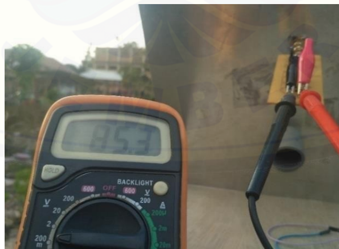
Figure 12. Testing of Energy Harvesting Rectenna
