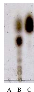
Figure 1. Result of thin layer chromatography (TLC) analysis of OPEFB-hydrolyzates. Ten percent dried-OPEFB with no buffer condition was digested by crude-enzyme 42 hours at 37°C. OPEFB-hydrolyzate with no enzyme as control (A), product (B) and glucose standards (C) was analyzed by TLC.
