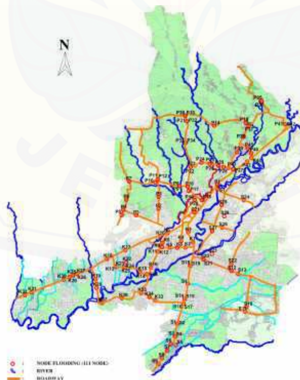
FIG. 4 Location of Nodes Flooding
