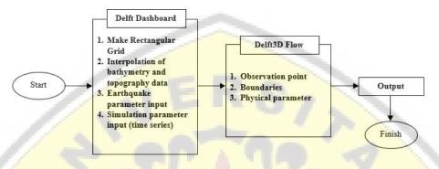
Figure 2. Framework of numerical modelling
