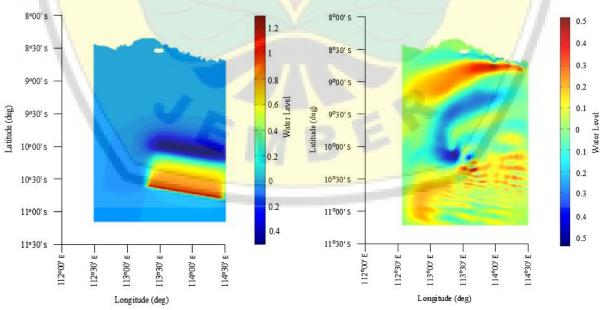
**Figure 3.** Initial surface elevation of Scenario 1
