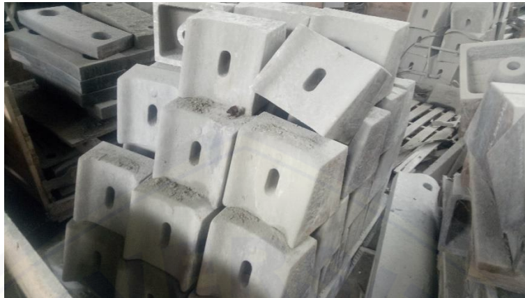
Gambar 2. 6 Liner (sumber: PT. XYZ tuban)
