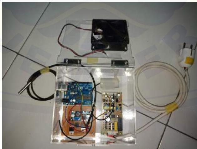
Gambar 3.5 Controller system pendingin MQL
