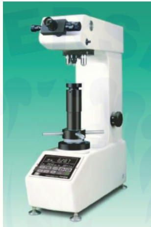
Gambar 2.5 Alat Vickers Hardness Tester (Sumber: Future-Tech Corp., 2015)
