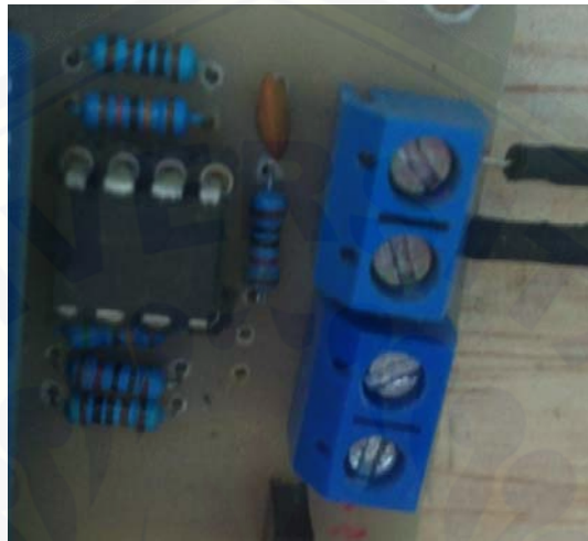
Gambar 3.5 Hasil Rangkaian Non Inverting
