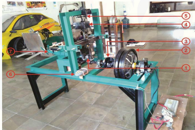
Gambar 2.18 Alat uji rolling resistance (Sumber: Kurniawan, 2017)
