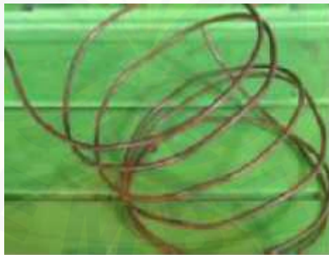
Gambar 2.6 Pipa kapiler (sumber :Stoecker and Jones, 1996)
