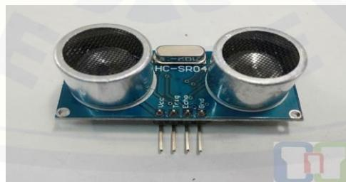
Gambar 2.5 Sensor Ultrasonik HC-SR04
