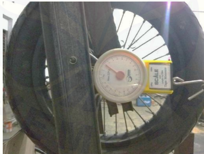
Gambar C.4 Pegas pengukur gaya tangensial
