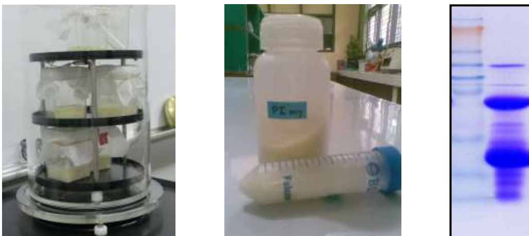
Gambar 3. A. Tahapan freeze dried protein isolate, B. Hasil protein isolate C. Profile SDS PAGE protein isolate
