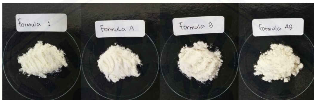
Gambar 4.1 Serbuk microspheres metformin hidroklorida formula (1) pengadukan 600 rpm, 2 jam; formula (A) pengadukan 1200 rpm, 2 jam; formula (B) pengadukan 600 rpm, 4 jam; formula (AB) pengadukan 1200 rpm, 4 jam.
