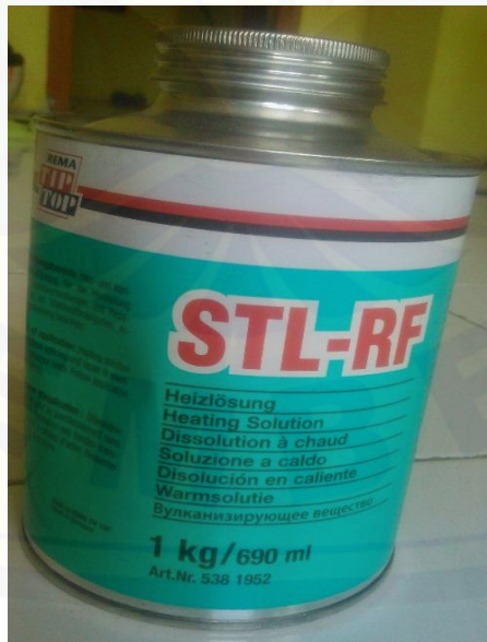
Lem hot splicing
