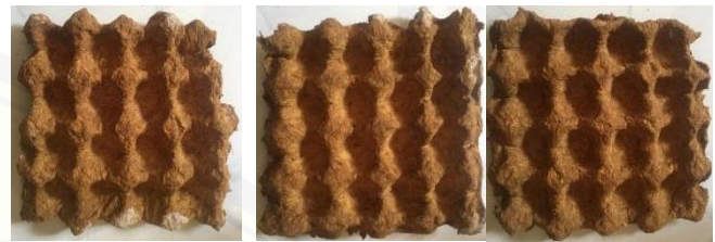
Figure 7. Eggs tray tobacco stems (a) NaOH 5 percent, (b) NaOH 10 percent, (c) NaOH 15 percent
