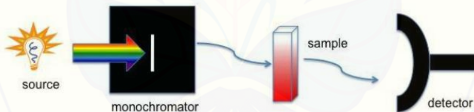
Gambar 2.13 Ilustrasi instrumen sinar-ganda UV-Visible (Shah dkk., 2015)
