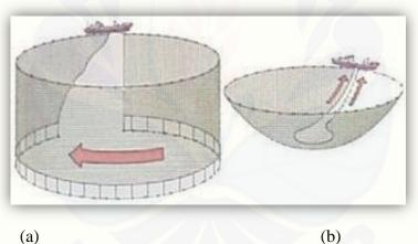
(b) Figure 1. How the slerek boat works Source : (a) www.kotaikan.blogspot.com (b) www.minapedia.online
