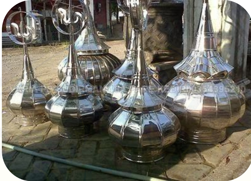
Gambar 1. Kubah Berbahan Stainless Steel (sumber: www.solusirumah.biz )
